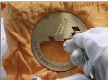
An employee sorts the edges of the Winter Olympic medal design at the ADAMAS jewellery factory. Each medal takes up to 18 hours to create and the latest design and technology processes are used in the manufacturing process.
